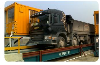
Kong and a significant world-wide sales volume. The design makes good use of appropriate materials such as compressed wood and concrete for a lower overall weight and easy transport, and reduces environmental impact since the instrument could be relocated when needed.
